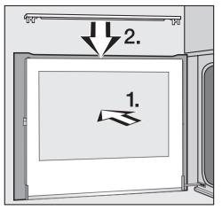
Refit the cover trim ②. As you do so press the inner pane ① to ease it into its groove in the cover trim.
